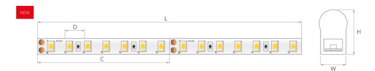
Dimensions: Width [W]: 0.2" | Max run length: 137.8" | Cut every [C]: 1.5" | Height [H]: 0.4"
